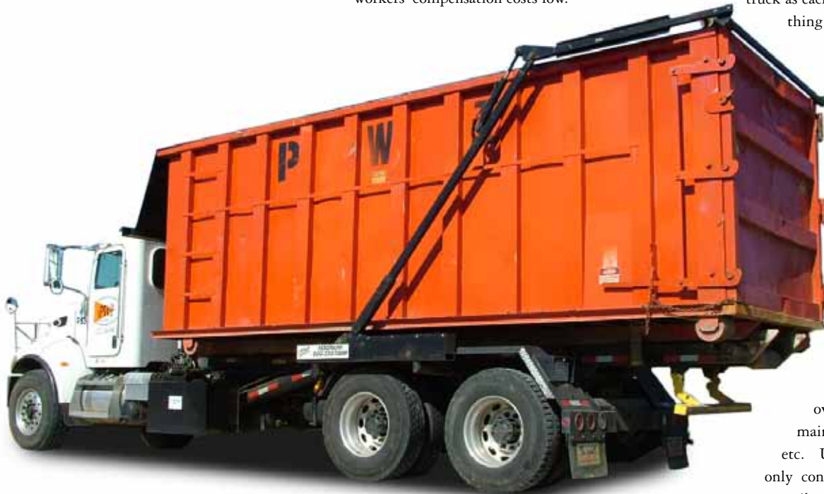
Magnum tarping system covering a 22' 40-yard box. Photos courtesy of O'Brian Tarping Systems.
