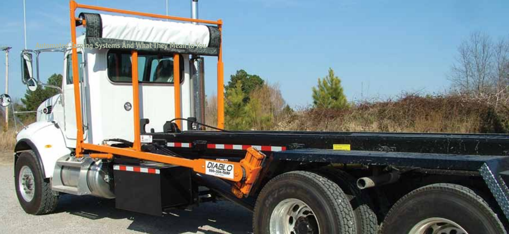
Diablo tarping system with the arms completely below and in front of the majority of containers and compactors.
