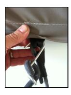
2. Remove all of the rubber straps from the trailer. Take the hook end and slide it back through the webbing that is sewn to the cover. This will minimize the hook from grabbing other hooks, cushions, etc and make installation easier
