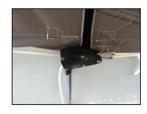
8. Take the rope ratchet and attach it to the looped end. Take the free end and feed it under and around the pawl. Pull tightly. You may need to physically pull the ratchet to the rear and retension if more tension is desired.
