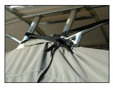
5. Install the Driver's side straps like the Pass side. This side, you can tension the straps to keep the tension OFF of the zipper. If you are straining to get the zipper started, release the tension from the Pass side and try again. Bring the zipper down to the edge of the boat.
