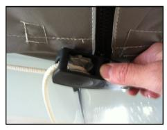
1. To release the tension on the ratchet, pull on the loose end of the rope and press the release latch with your thumb. This will allow the ratchet to free wheel. Pull all of the rope out of the ratchet, remove the ratchet from the looped rope and set aside for later
