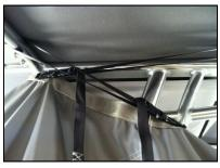
4. Install the two straps on the Passenger side. The front strap will run to the rear, around a bar and back to itself. The back strap will be the exact opposite. Do NOT overtension this side before tensioning the drivers side or zipper damage will occur!
